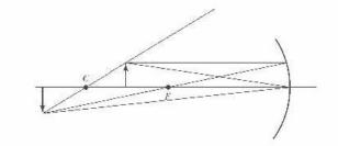
b)  $\frac{1}{s} + \frac{1}{s'} = \frac{1}{f} \Rightarrow \frac{1}{s'} = \frac{2}{22.0 \text{ cm}} - \frac{1}{16.5 \text{ cm}} \Rightarrow s' = 33.0 \text{ cm}$ , to the left of the mirror.  $y' = -y\frac{s'}{s} = -(0.600 \text{ cm})\frac{33.0 \text{ cm}}{16.5 \text{ cm}} = -1.20 \text{ cm}$ , and the image is inverted and real.
